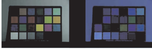
Figure 4. Macbeth color checker under different illuminant. (a) Phillips Ultralume fluorescent tube (b) Solux 3500K +Roscolux 3202 blue filter [17].
